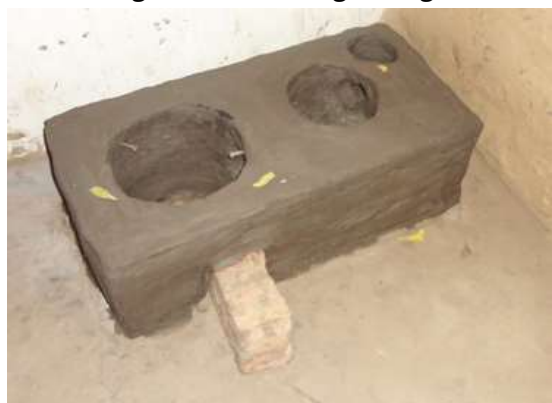
Newly smoke-less Chula using iron frame, made by trained woman in Zarda
